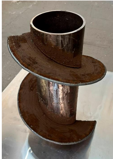
Figure 4. Appearance of the surfaced fragment of the auger
