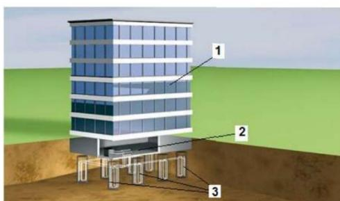
*Fig. 2. The general layout of the building's elements heated with the use of energy piles:
