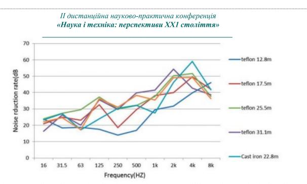
Fig. 1. Rate of sound attenuation (dB) in octave frequencies at different distances in simulated ear canal
