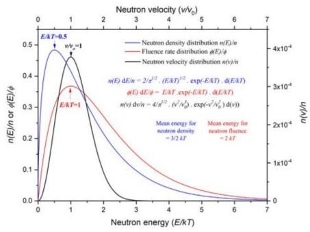
Fig. 1. The thermal Maxwell–Boltzmann distributions in energy, fluence and velocity.
