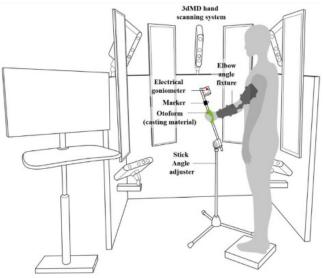
Fig. 2. Experimental layout for palmar hand dimension measurement.
