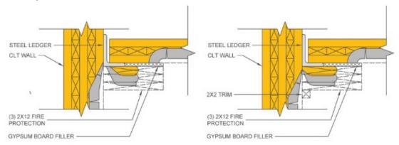
Fig. 2. Effects of Char Contraction on Differently Protected Steel Ledgers
