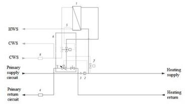
Figure 1. Schematic diagram of the EvoFlat FSS.
