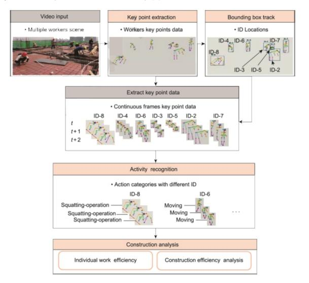
Figure 1. The framework of multiple worker construction actions and working efficiency recognition.
