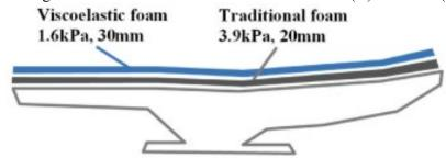
Fig. 2. Side view diagram of seat prototype in flat condition.
