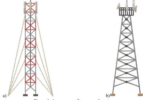
Figure 1. Appearance of towers and masts. a) mast b) tower
