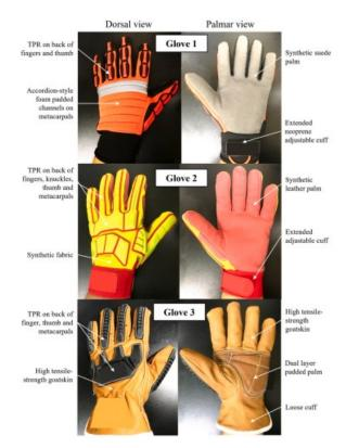
Fig. 1. Industrial metacarpal gloves selected for testing. All branded labels have been intentionally removed from the figure to prevent bias. The gloves are presented from thinnest (Glove 1) to thickest (Glove 3).
