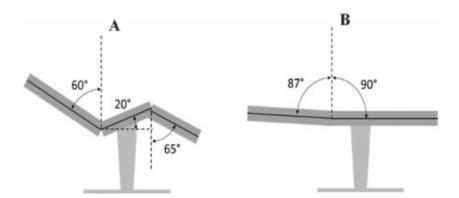
Fig. 1. Configurations for reclined and flat seat conditions. (A) Reclined (B) Flat.
