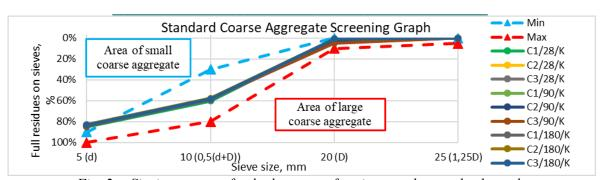
Fig. 2. Sieving curves of only the coarse fractions on the standard graph.
