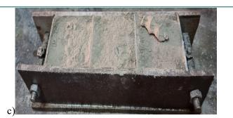
Fig. 1 Production of soil concrete specimens with dimensions of 70x70x70, using recycled products: a) cubes; 10% aggregate content; b) 20% aggregate content; c) 30% aggregate content.
