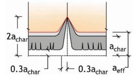
Fig. 1. Char Contraction at Unbonded Abutting Wood Members
