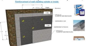
Pic 3. Scheme of MAPEI FRG amplification system [3,4, 6]
