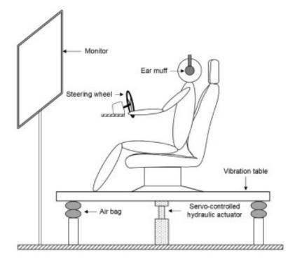
Fig. 1. The schematic diagram of the setup in the laboratory.
