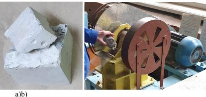
Fig. 1.a – the split sample a cracked sample of source concrete without structural disturbance; b – laboratory jaw crusher with complex rotation.
