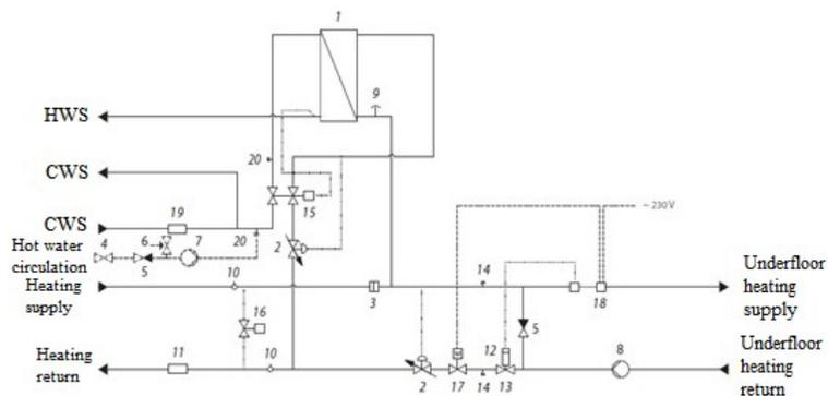
Fig. 2. Schematic diagram of the EvoFlat 4.0 M.
