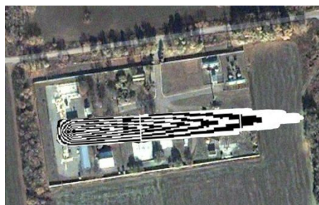
Fig.6 Polluted area at ammonia-pump station, t = 15s
